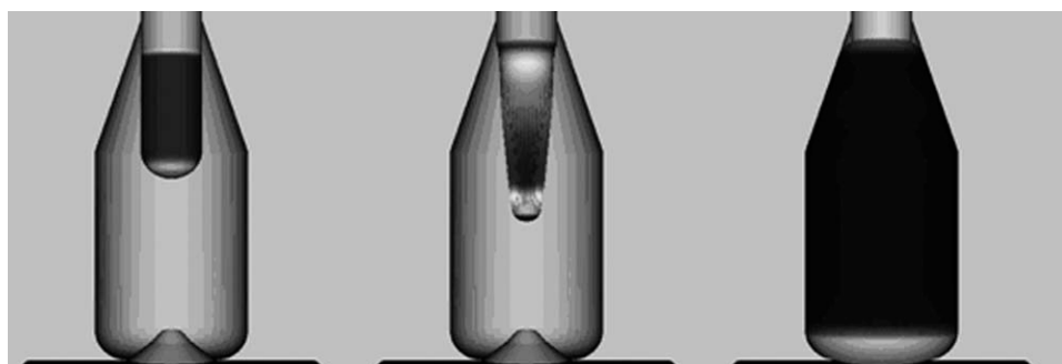
Figure 4 Preform deformation steps—Model 2.
